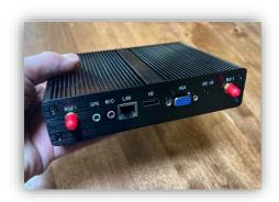
**STREAMBOX:** Locate in a cool place with good air circulation. Do not put on top of warm equipment.
